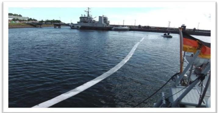
German Navy Kiel: Schucu oil absorbing barrier belts, 25m each
